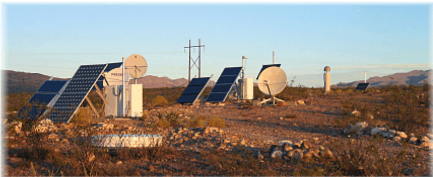
EarthScope prototype seismic stations being tested at New Mexico Tech
