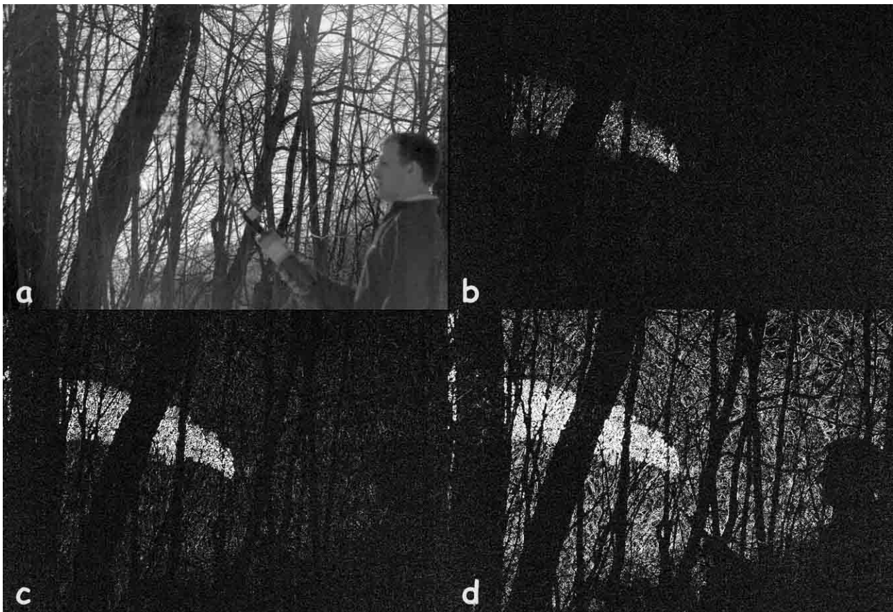
Fig. 3 Images showing torch plume visualized against a background of trees trans-illuminated by the afternoon sunlight. The original image (a) is compared to images taken 0.667 ms (b), 2 ms (c), and 10 ms (d) later.
