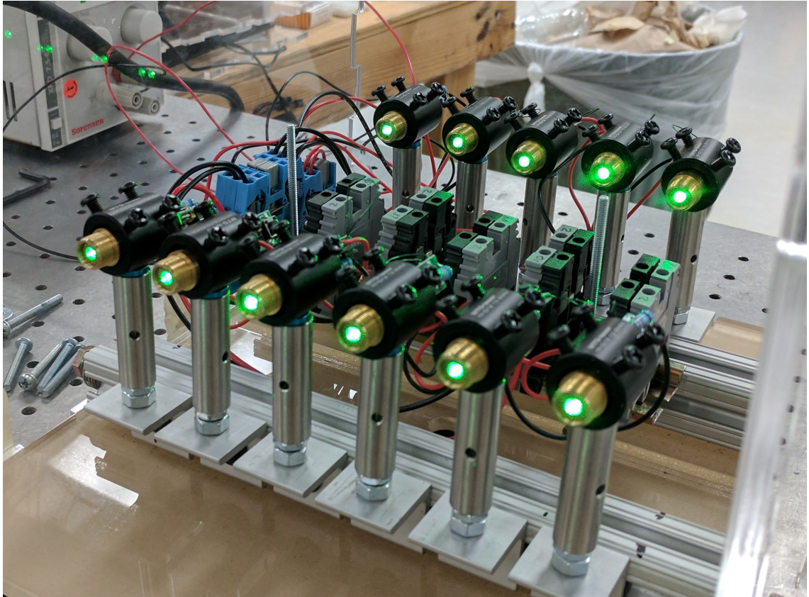
Figure 2.3: The staggered placement of laser positions to allow the formation of a singular light sheet.
