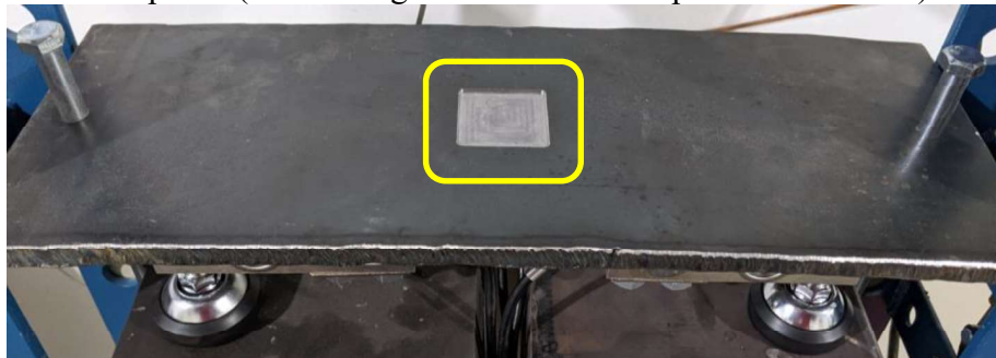
Figure 1: Guide rods in place and pressing surface aligned with bottom bed holes. Yellow outline indicates alignment groove location.
