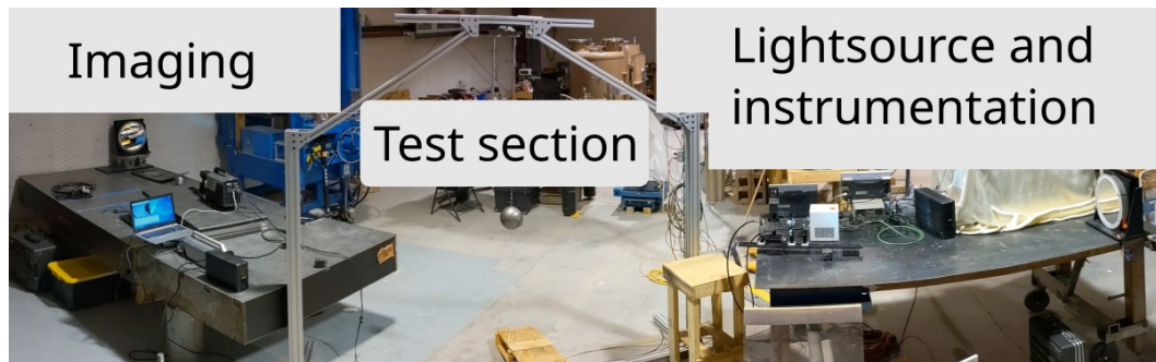
Figure 2.1: Alignment setup for Z-type schlieren
