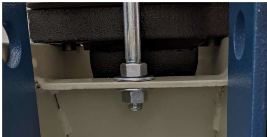
Figure 2: Side view of guide rod once secured to bottom bed and rod fed through holes in scale bed.
