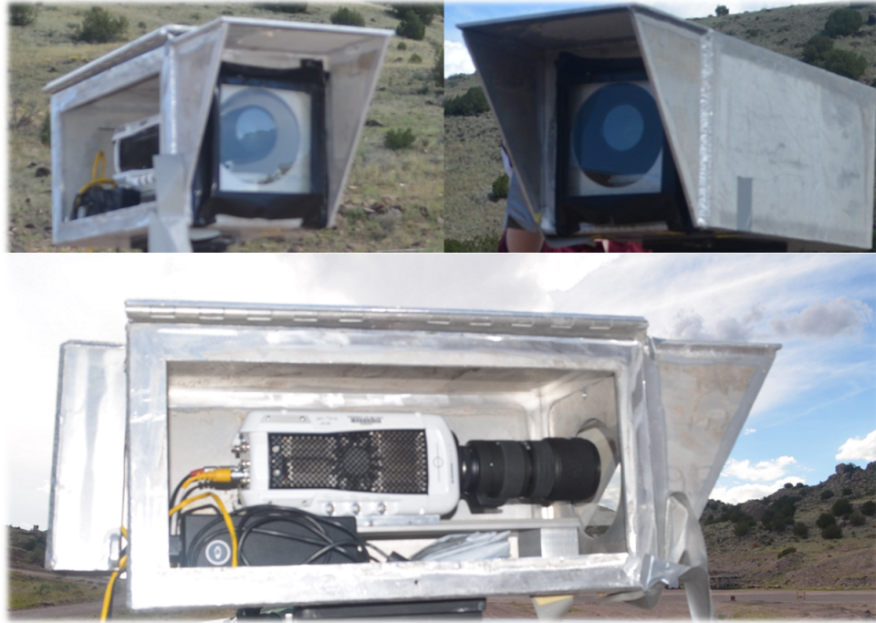
Figure 2.2: Aluminum Box of 0.25" thick plates protecting the Phantom v711 high-speed camera.
