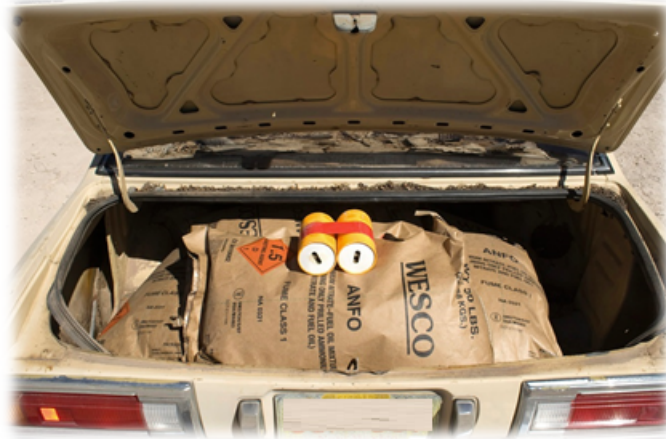
Figure 2.8: General placement of charges inside the trunk of a car
