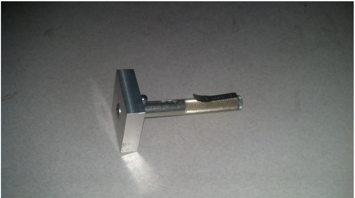
Figure 2.8: Firing mechanism and holding block
