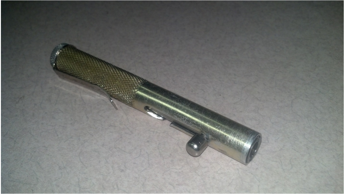
Figure 2.7: Shotgun shell primer firing mechanism
