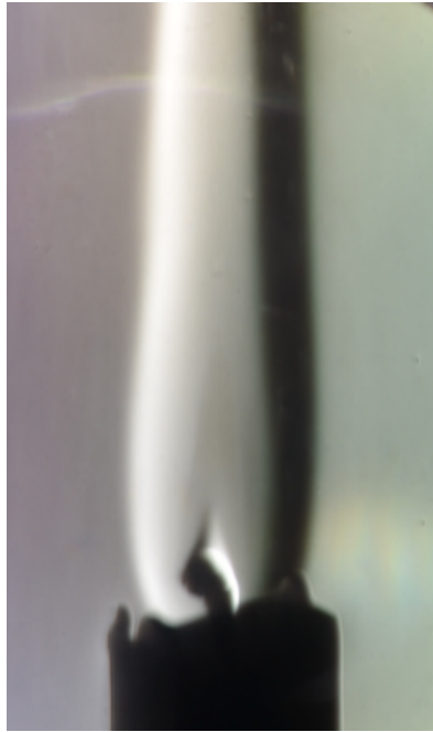
Figure 2.3: Photo of candle using schlieren imaging technique
