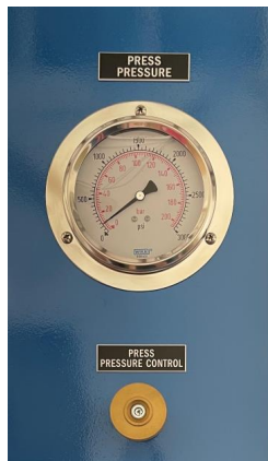
Figure 7: image of the press pressure gauge and the control valve.
