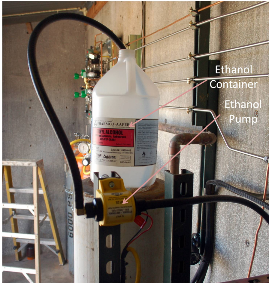
Figure 4.13: Ethanol pump connected to ethanol source container
