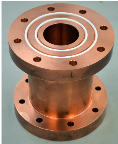
Figure 3.5: Completed combustion chamber with o-rings installed
