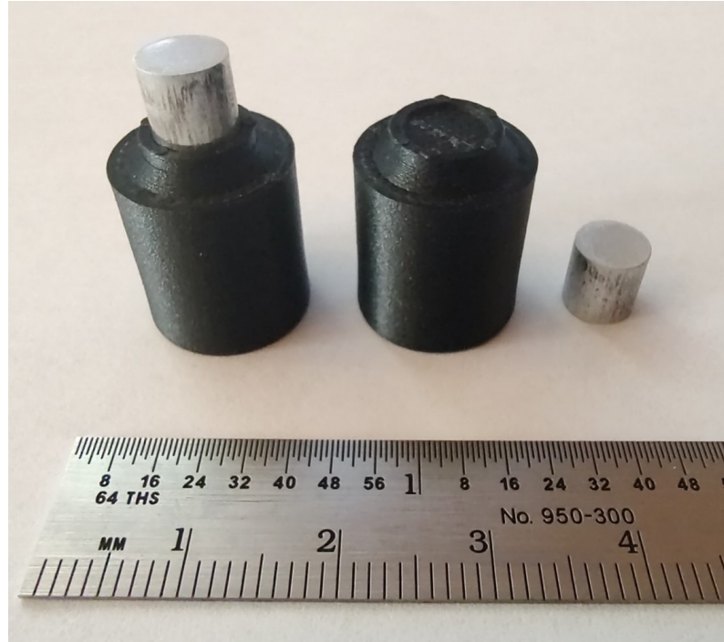
Figure 3.8: Example of additively manufactured sabots with RM cylindrical specimens. At left is a sabot with RM specimen installed in preparation for launch in the 14 mm powder gun. At right is the sabot and specimen separated prior to assembly. The ruler scale is marked in millimeters on the bottom and inches on the top.
