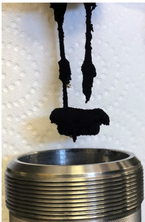
Figure 8.3: Soot formation in Parr 1108 bomb resulting from the Al/PTFE reaction.
