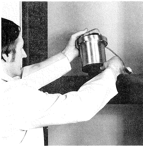
Figure 5-10. Installing a Tension Cell in the Moving Crosshead
