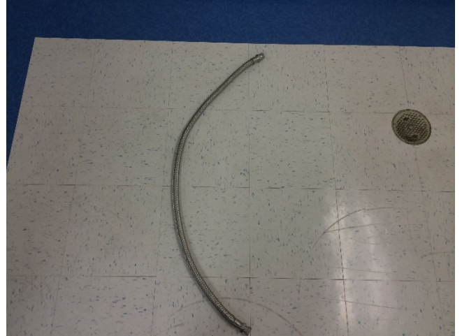
Figure 11: Nitrogen Transfer Hose.
