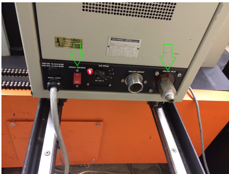
Figure 6: This is the back of the ECC. On the left is the power switch. On the right the Coolant Inlet, where the liquid nitrogen transfer hose is connected.
