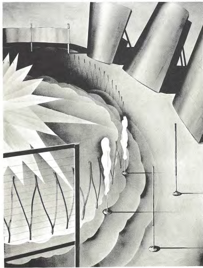
ARENA DETAIL DATA-TAKING BY FIRING AGAINST WIRE SCREENS, FLASH TUBES, PATTERN SHEETS AND AIRCRAFT STRUCTURE
